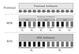
Fig. 1. HPR seen as trade-off between positional and RNS representations.
