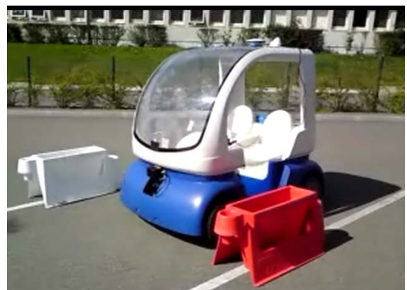
Fig. 1. The automatic CyCab vehicle developed at INRIA equipped with odometers, DGPS, and laser range finder
