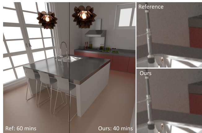
Figure 3: Interior scene rendered with 10000 paths/pixel, 4 diffuse/glossy bounces and 24 transmissions bounces using a sobol sequence. The reference image was generated using a classic Cranley-Patterson de-correlation method. The image referenced as "ours" was generated using our micro-jittered sampling technique. Both rendering times are reported from a NVIDIA 980Ti GPU.
