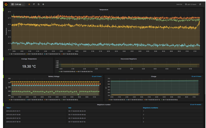
Fig. 4: Example dashboard for visualizing sensor the measurements and network statistics from the Inria Smart Building pilot deployment in real time.
