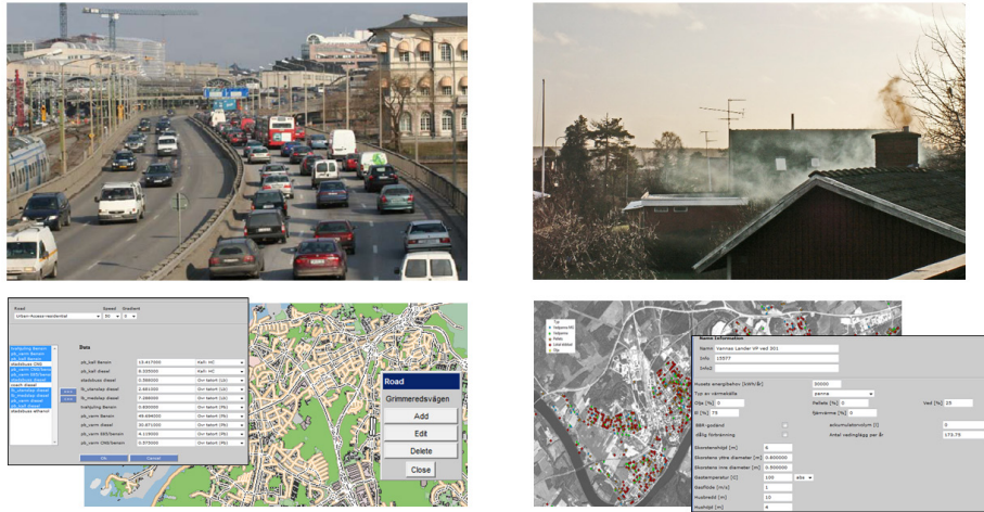
Fig. 2. The two major sources to PM 2.5 pollution in Sweden and how the GUIs of the Airviro Emission Database can be used by local end-users to modify/update information of mobile sources (left) and residential wood combustion sources (right).
