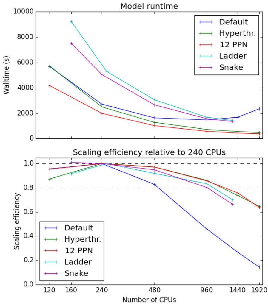
Fig. 3. Model walltime (a) and scaling efficiency (b)
