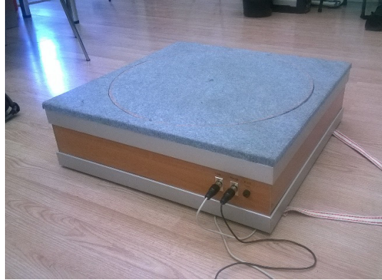
Fig. 2. The Arduino based scan turntable designed and constructed at Biotech Laboratory for 3D body scanning.
