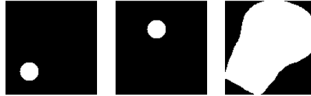
Fig. 4. A segmentation object containing two markers. Image processing “merged” the two nuclei into one segmented object.
