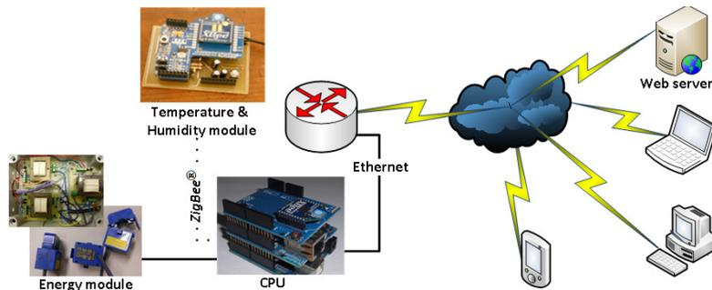
Fig. 3. Developed prototype of a web-based meter
