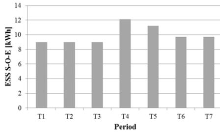
Fig. 5. ESS State-of-energy during the time horizon.
