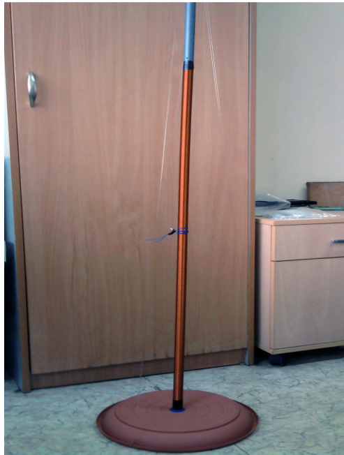
Fig. 1. Example of poorly constructed quarter-wave resonator coil.
