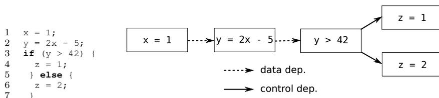
Fig. 1: A code snippet and its PDG
