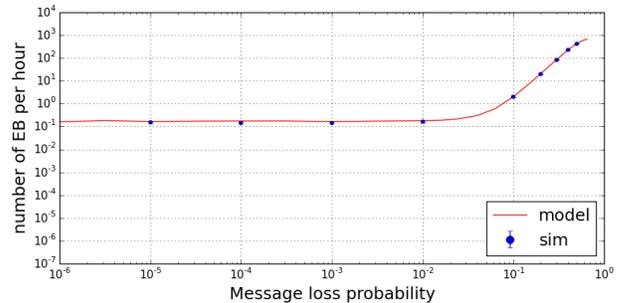
Figure 8: Number of emergency brakes per hour.
