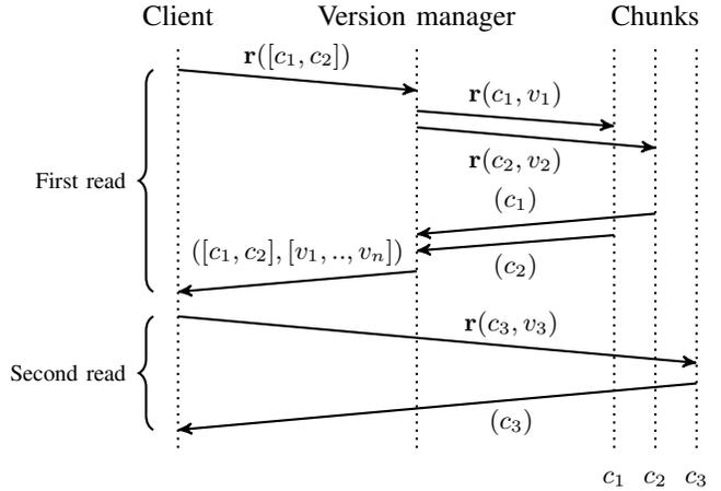
Fig. 4. Týr read protocol inside a transaction. The client sends a read query for chunks  $c_1$  and  $c_2$  to the version manager, which relays the query to the servers holding the chunks with the correct information, and responds to the client with the chunk data and a snapshot of the chunk versions. Subsequent read on  $c_3$  is addressed directly to the server holding the chunk data using the received chunk version information.
