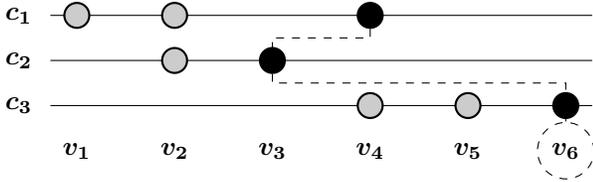
Fig. 3. Version management example. The version  $v_1$  of this blob only affected the chunk  $c_1$ ,  $v_2$  affected both  $c_1$  and  $c_2$ . In this example,  $v_6$  is composed of the chunk versions  $(v_4, v_3, v_6)$ . This versioning information is stored on the blob's metadata nodes.
