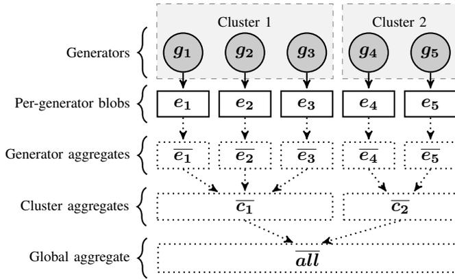
Fig. 1. Simplified MonALISA data storage layout, showing five generators on two different clusters, and only three levels of aggregation (*generator*, *cluster*, and *all*). Solid arrows indicate events written and dotted arrows represent event aggregation. Each rectangle indicates a different blob.
