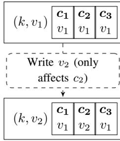
Fig. 2. Týr versioning model. When a version  $v_2$  of the blob is written, which only affects chunk  $c_2$ , only the version of both the blob and  $c_2$  is changed. The version id for both  $c_1$  and  $c_3$  remains unchanged.
