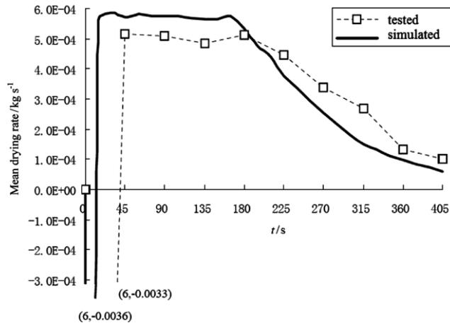
Fig. 5. Drying rate curve of rapeseed from simulation and experiment
