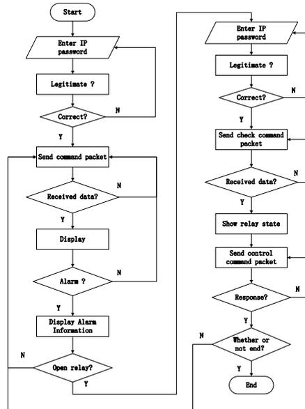
Figure 4 Facilities environment monitoring system flowchart
