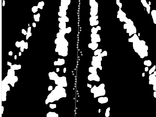
Fig. 9. The detected Navigation Line
