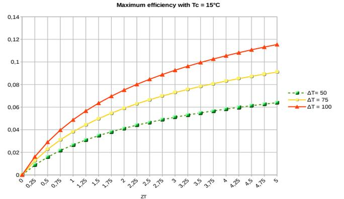
Fig. 2: Maximum TEG efficiency in the supercomputer scenario
