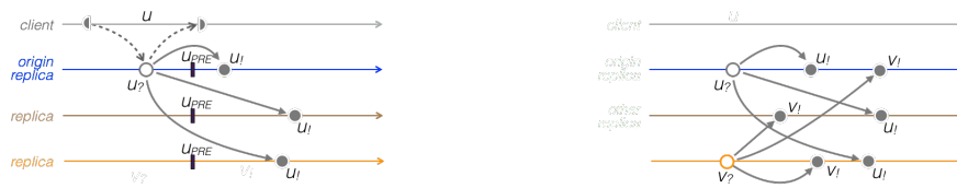
(a) Operation u decomposed into indivisible call, return, generator u_g and effector u_l . Precondition u_{PRE} is true at the effector. (b) The effectors of concurrent operations may execute in different orders in the general case.
