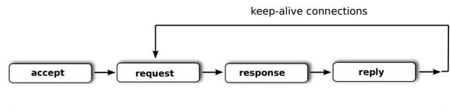
Figure 4. Internal pipeline of the Hop web server.
