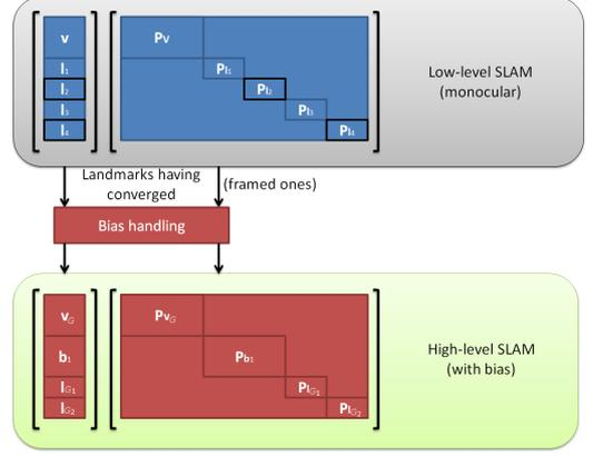
Fig. 1. Architecture around the bias estimation
