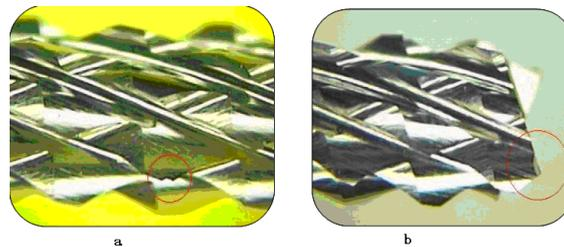
Fig. 4. Missing angle with (a) Middle edge missing angle and (b) Fish tail edge missing angle
