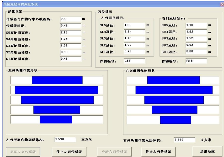
Fig. 9. The working screen capture of orchard measurement system of canopy volume.
