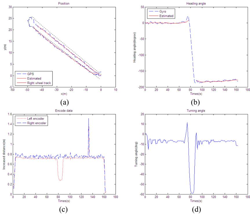
**Fig. 3.** Experiment data by drawing line on ground, (a)original GPS position, estimated position and track of right wheel; (b) original gyro data and estimated heading angle; (c) left encoder and right encoder data; (d) turning angle sensor data
