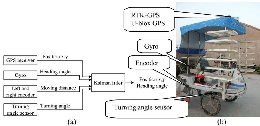
**Fig. 1.** (a) configuration of the multi-sensor system; (b) the test platform on the ISEKI ZP60
