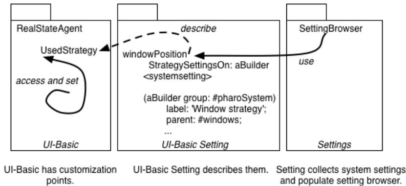
**Figure 5.** A package declares and uses customization points as variables. As an example, *UsedStrategy* is declared as a class variable of *RealEstateAgent*. Such customization points are described with *Setting* instances that are created by the automatic running of setting declaration methods. The *Setting Browser* collects the setting instances by querying pragmas and presents them to the user.
