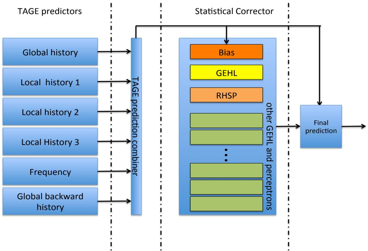
Figure 1: Prediction computation flow on the MTAGE-SC predictor
