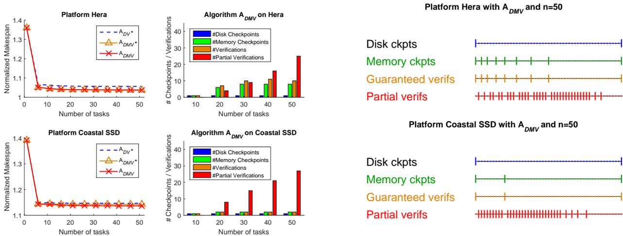
Figure 7. Performance of the three algorithms, and distribution of disk checkpoints, memory checkpoints and verifications (for the  $A_{DMV}$  algorithm) on platforms Hera and Coastal SSD with the *Decrease* pattern.
