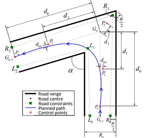
Fig. 1. Curve representation on an intersection scenario
