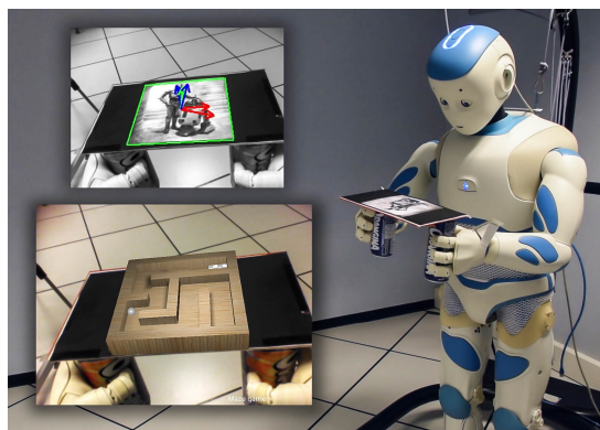
Figure 1: Romeo solves a ball-in-maze game in augmented reality using two hands. Only vision is used to control both arms.
