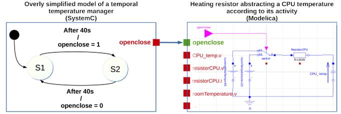
Fig. 4. A simple example mixing SystemC and Modelica
