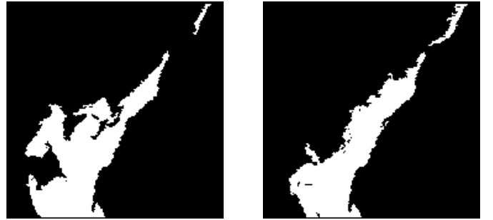
Fig. 3: Extracted upwelling areas using the region-growin algorithm over the two binary images of Fig. 2
