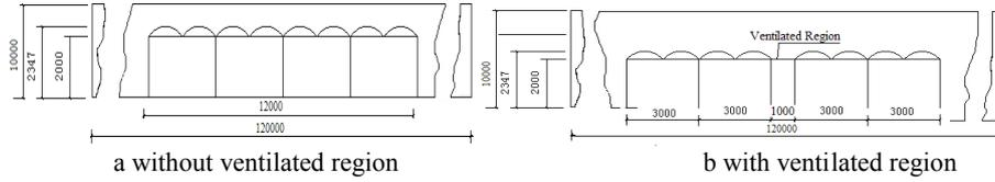
**Fig. 1.** Schematic diagram multi-span grape rain shed (mm)
