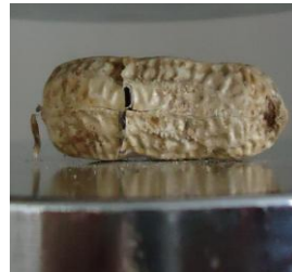
(b) Cracking transversely
