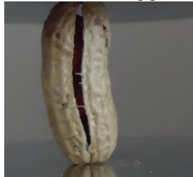
(a) Cracking longitudinally
