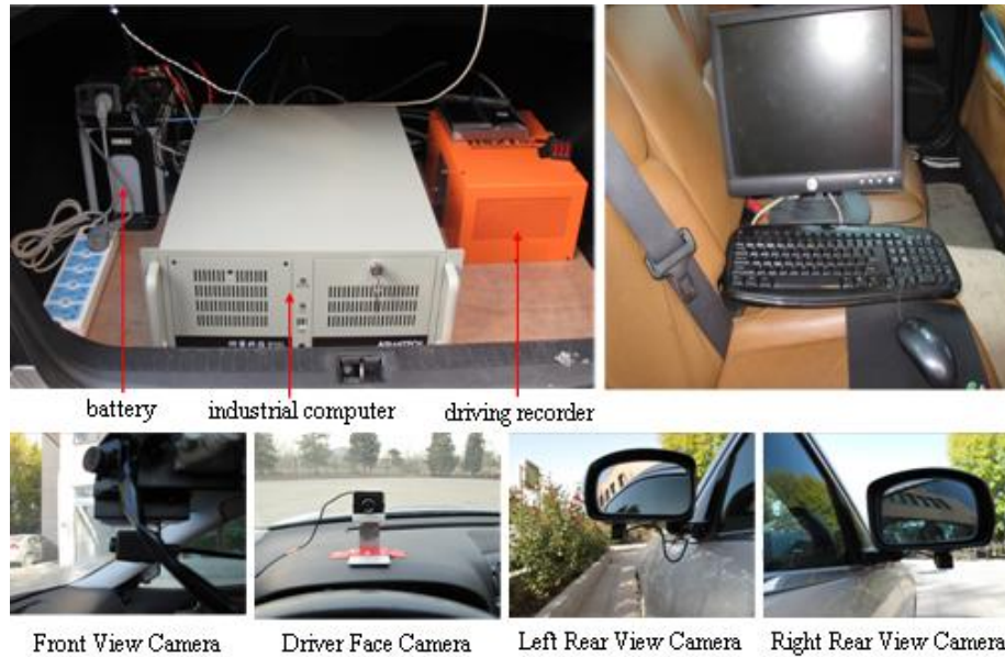
Fig.1. Data acquisition system
