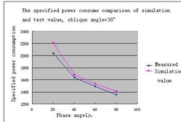
**Fig.10.**The specified power consume comparison of simulation and test value, oblique angle=30°
