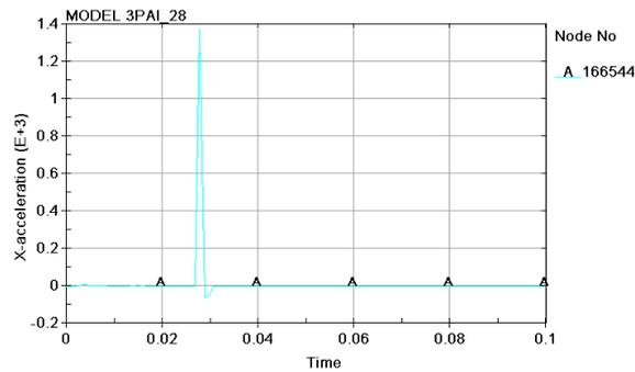
**Fig. 5.** The acceleration of soil element no.166544
