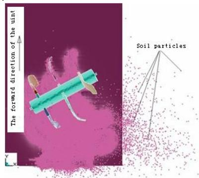
**Fig.13.** Throwing Soil simulation of oblique rotary tilling
