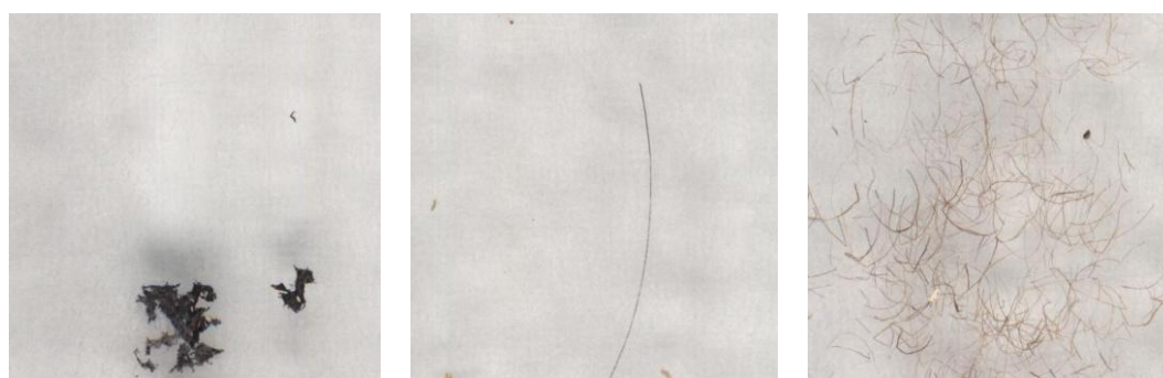
Fig. 3. Acquired color image examples: (a) opened plastic film, (b) opened hair, and (c) opened hemp rope.
