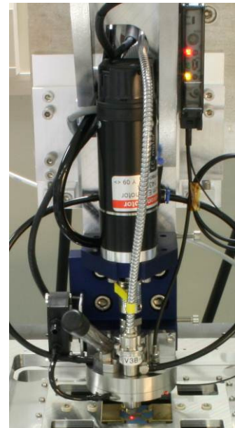
Figure 7: bond head in assembly environment
