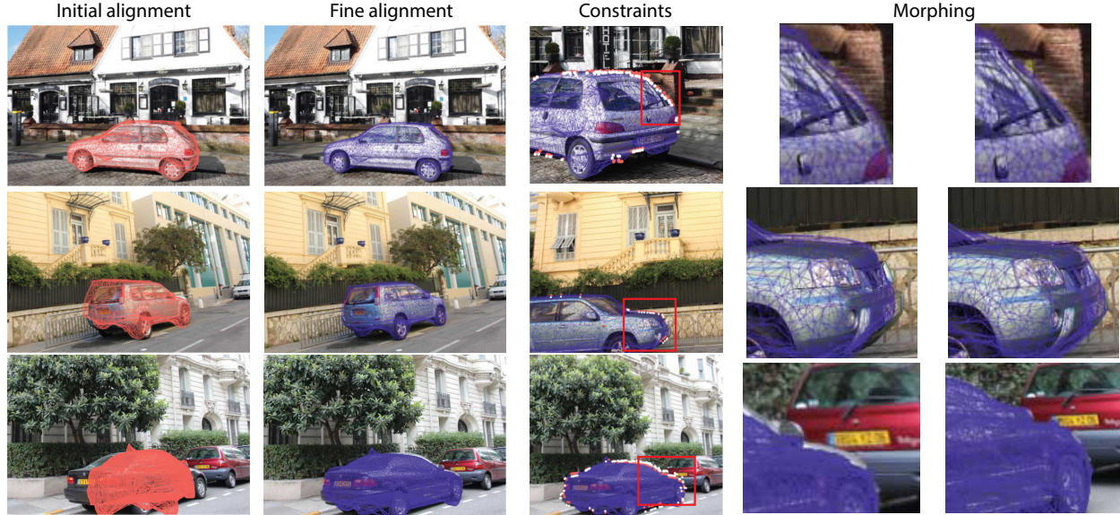
Figure 8. Mesh alignment and morphing. (a) Using 2D detection bounding boxes, an initial transformation of the 3D model is computed. (b) Using available 3d reconstruction and constraints from silhouette matching, a fine grain alignment of the model is estimated. (c) Because the 3d model does not always correspond to the images, deforming the mesh is necessary. Red points indicate mesh vertices to be displaced. White points indicate their target position. (d&e) After morphing, we obtain a better alignment of the 3d model.
