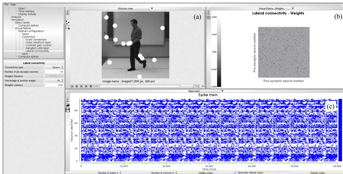
Figure 5: Spike generation from our retina simulator. (a) Input image sequence with spiking activity super-imposed (white blobs). (b) Connectivity matrix chosen for the simulation, here random. (c) Simulated spike train.
