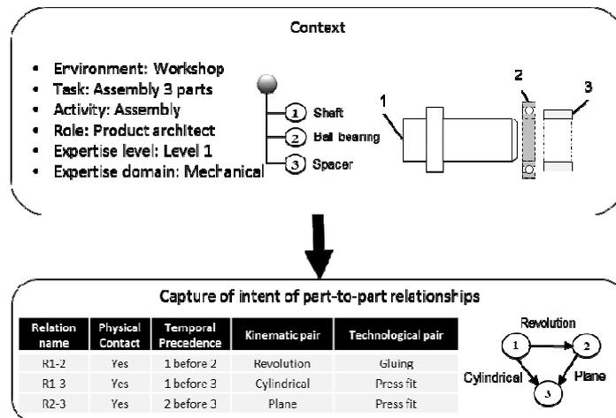
Fig. 3. Capture of design intent through part-to-part relationships
