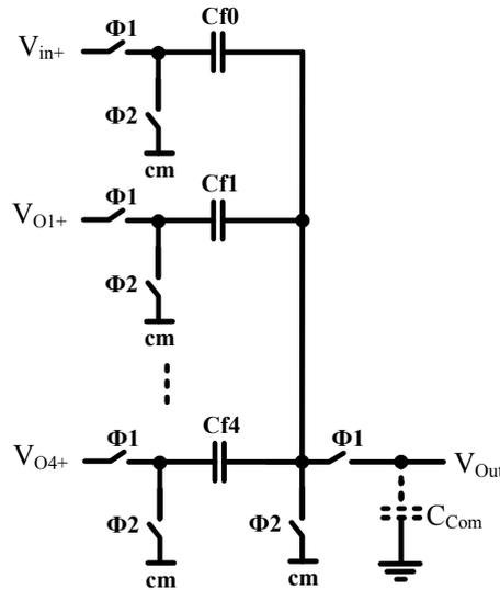
**Fig. 16.** Passive adder. Single-ended scheme is shown for the sake of simplicity.  $V_{oi+}$  ( $i = 1-4$ ) is the  $i$ -th integrator's output, and  $C_{Com}$  represents the parasitic capacitor at the input of the comparator
