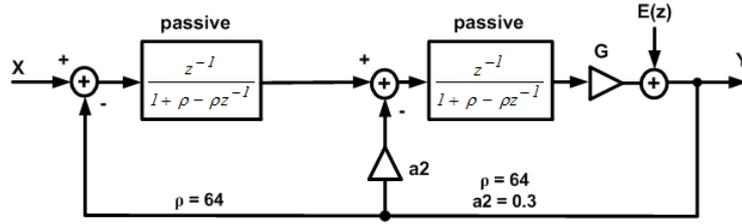
Fig. 1. The linearized model of the 2<sup>nd</sup>-order passive  $\Delta\Sigma$  modulator using distributed feedback topology [7] (Courtesy of IEEE)
