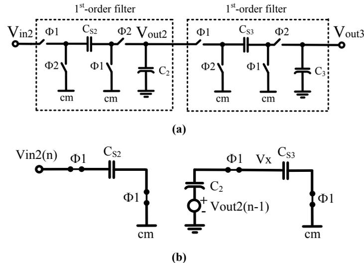
**Fig. 12.** (a) A 2<sup>nd</sup>-order passive low-pass filter built from the cascade of two basic passive filters, (b) Equivalent model in sampling phase  $\Phi 1$
