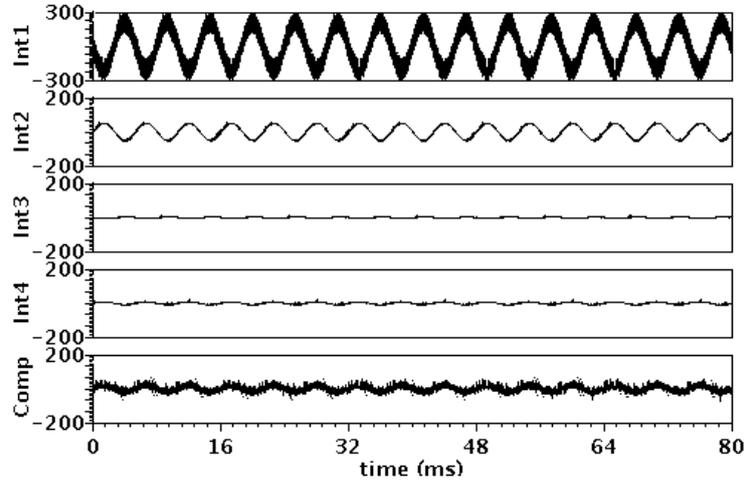
**Fig. 7.** Integrators output swing in mV using a -1.94 dBFS, 187 Hz input signal. Comp represents the comparator input signal, and *Inti* ( $i = 1-4$ ) represents the  $i$ th integrator output [7] (Courtesy of IEEE)
