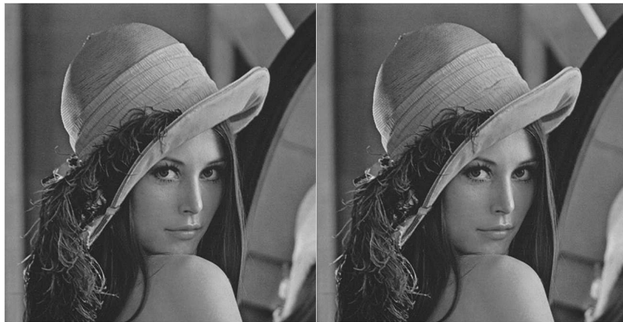
(a) Floating-point IDCT, compression rate=2.3 (b) Fixed-point IDCT, compression rate=2.3
