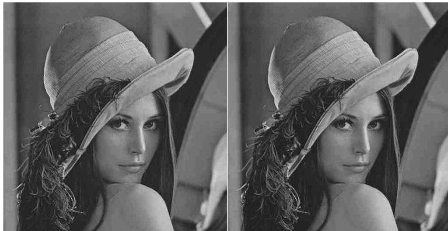
(c) Floating-point IDCT, compression rate=45 (d) Fixed-point IDCT, compression rate=45
