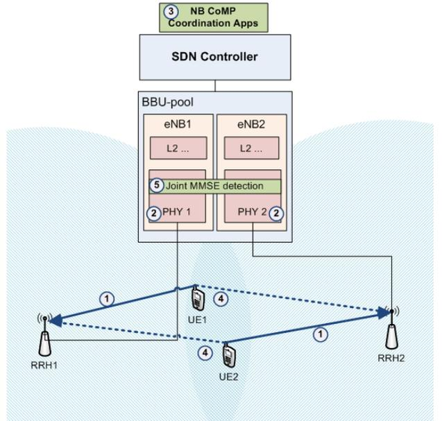
Fig. 2. Uplink joint detection architecture and coordination process
