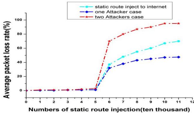
Fig.6. Packet Loss Rate Trend
