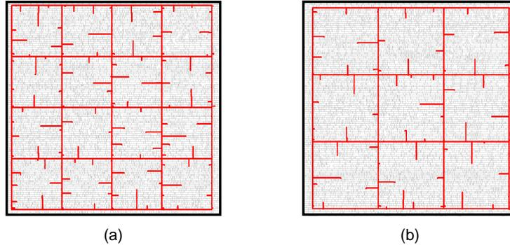
Fig. 10: Layouts of single-mesh networks of different postmesh structures.
