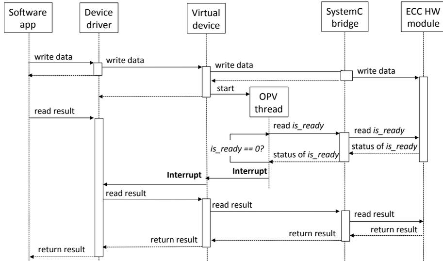
**Fig. 8.** Sequence diagram of the interrupt mechanism for ECC benchmark.
