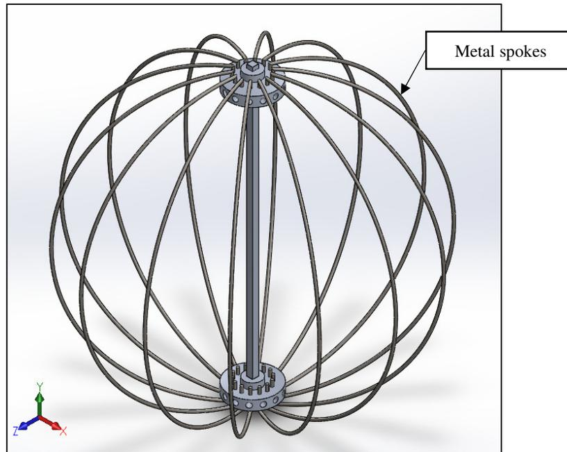
**Fig. 1.** The proposed design of spherical mobile robot
