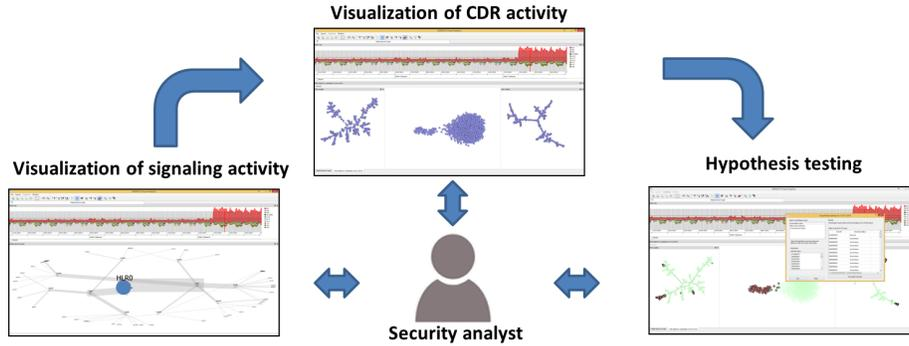
**Fig. 2.** Overview of the proposed visual analytics tools integrated in MoVA. An overview of the network is provided to the analyst by visualizing aggregated signaling activity. Reducing the abstraction level, CDR data of specific users are used to visualize their behavioral similarities. Finally, the analyst can formulate and test specific security-related hypotheses.
