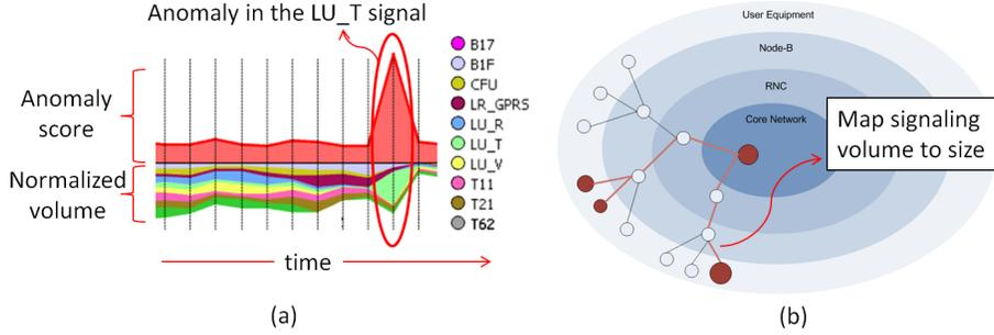
**Fig. 3.** Visualization of the signaling activity in the network. (a) Stacked graphs visualization of the anomaly scores and signaling volume. (b) A scheme of the proposed layered layout of the Mobile Network Graph.
