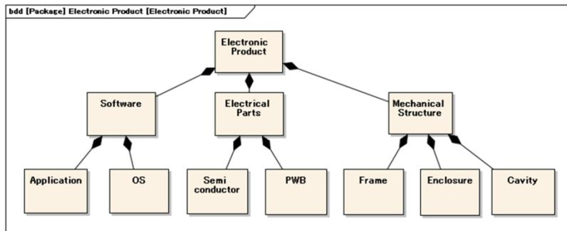
**Fig. 1** Diagram of modules in an electronic product
