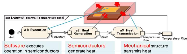
Fig. 3 Temperature rise in an electronic product
