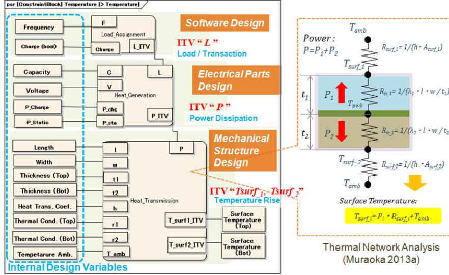
Fig. 5 Parametric model to simulate the temperature rise
