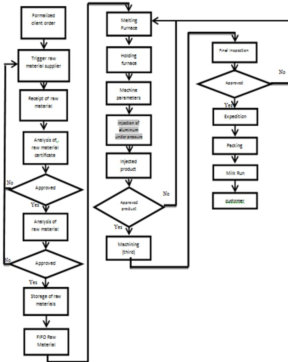
Figure 3: Flow of the customer order-to-delivery process
